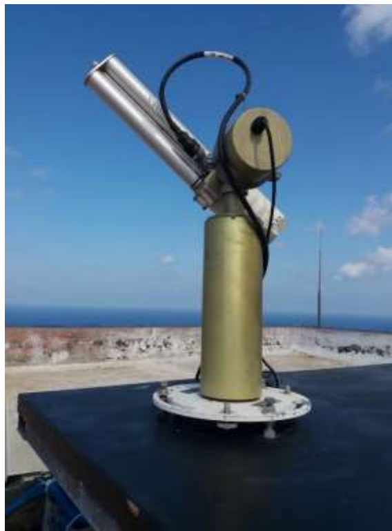
Figure 22: Photo of the CE318 photometer installed at the Antikythera Observatory. The platform has been painted black to avoid reflections.
